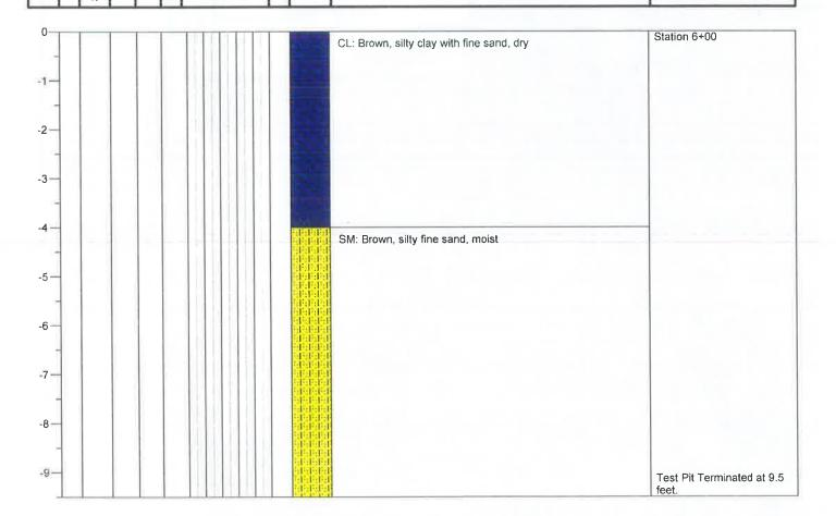
**TEST PIT NUMBER** Neil O. Anderson & Assoc., Inc. **LOG OF TEST PIT** 902 Industrial Way, Lodi, CA 95240 TP-2 (209)367-3701 Fax (209)333-8303 DATE EXCAVATED: 8-8-07 PROJECT NUMBER: LFG-0229 PROJECT NAME: Twitchell Island GROUND SURFACE ELEVATION: 0.0 Feet LOCATION: Sacramento County, CA PLATE NO. 3 Case Backhoe with 30 inch Bucket DRILLING EQUIP.: Sampling Method Ground Water Dry Density, Blow Counts Soil Lithology Depth, ft. Blow Count
